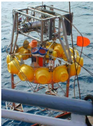
Exact positioning on the seafloor is carried out by the video-controlled Launcher
