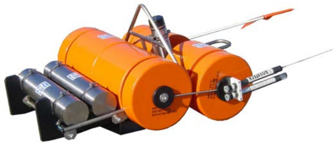
Lobster-6000 Longterm (side view) with two titanium pressure tubes (electronics tube, battery tube) + shock protection
