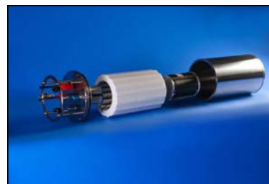
Data Logger, battery pack and seismometer in titanium pressure tube
