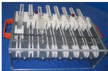
Rear view: 6 syringes in neutral position, 1 poison syringe, 1 drawn up syringe
