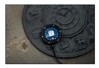
UHURA is connected to the distribution box DIRC and operated either over the accumulator or an USB connection. NMEA-strings with 4800 and 9600 baud are put out, in addition also the second pulse. The DCF77-signal is modulated on the second pulse so that the highest possible number of instruments can be provided.
