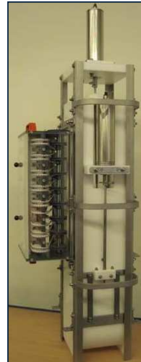
Benthic Chamber with Syringe Sampler
