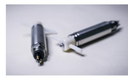
When performing some critical sample measurements on the seabed, it is important that collected samples are thoroughly mixed to ensure a constant concentration throughout the solution. To ensure that subsea samples can be mixed efficiently in situ, K.U.M. developed the Stirrer.
