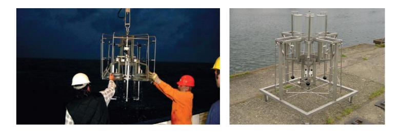
In many marine investigations, core samples are essential for ascertaining the bulk properties of underlying sediments, but obtaining these cores from the seabed with conventional multi-corers can be very challenging.
