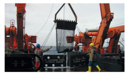
Samples of rock, nodules or cobbles from the seabed can provide geologists with valuable insights into the underlying strata and its properties. To obtain these samples efficiently and safely, K.U.M. developed the Chain Bag Dredge.
