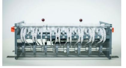
Scientific investigations that are easy in the lab are not so straightforward when they need to be conducted in the subsea environment with pressures of up to 600 bars. Our extensive range of products is designed to address these challenges, and the K.U.M. Syringe Sampler is an important addition.
